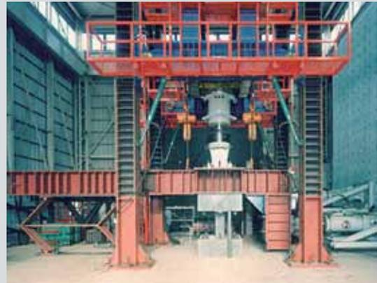
Structural testing of superhigh-strength RC columns
